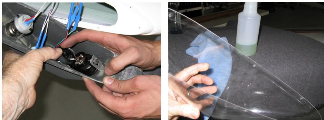
Reinstall the light terminal using the six sheet metal screws. Clean the wingtip cover inside and out with a mild cleaning solution (such as a spray bottle of water with just a few drops of Dawn) and a microfiber cloth. Reinstall the wingtip cover with the six sheet metal screws.
