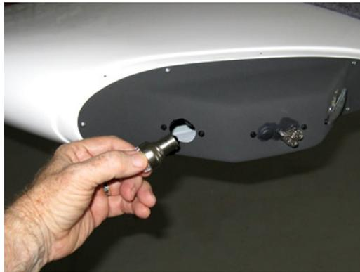
The position light bulb can be removed and replaced at this point. To remove the bulb, push gently and give it a counter-clockwise 1/4 turn, then pull it out. Replace the new bulb with a twist in the opposite direction.
