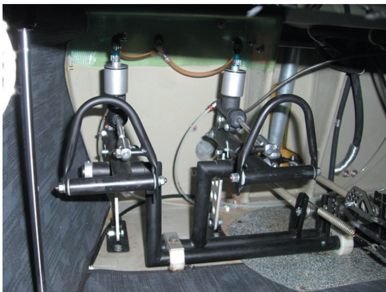
Pilot side installation complete.
