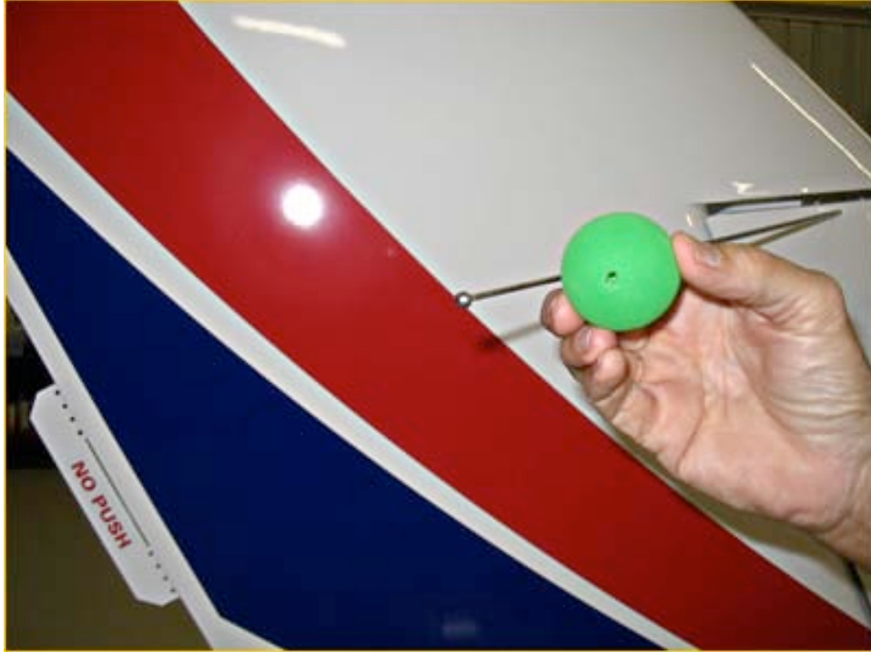
HOLE DRILLED HALFWAY THROUGH RUBBER BALL
