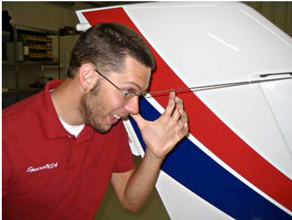
VOR/ILS ANTENNAE ARE ROUGHLY AT EYE LEVEL (BOTH SIDES OF RUDDER)
