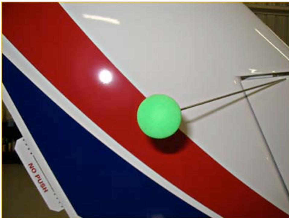
BALL PLACED OVER ANTENNA TIP (BOTH SIDES)
